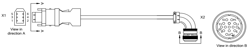
Figure 4-10 Absolute encoder motor wiring
