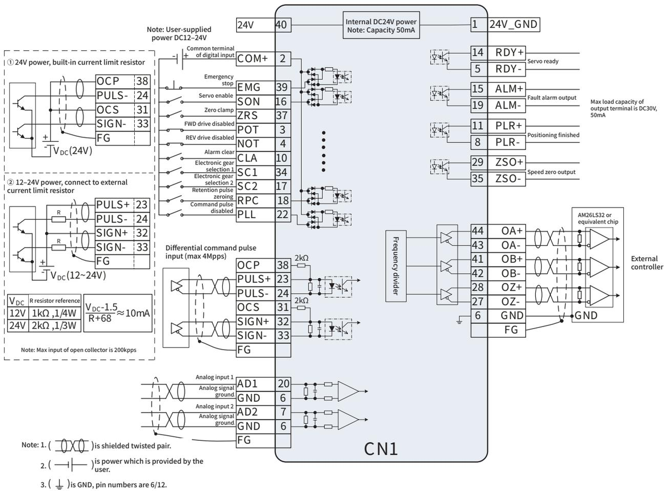
**Standard wiring diagram of speed mode
