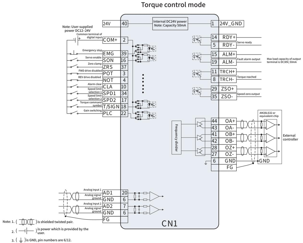
Standard wiring diagram of bus mode
