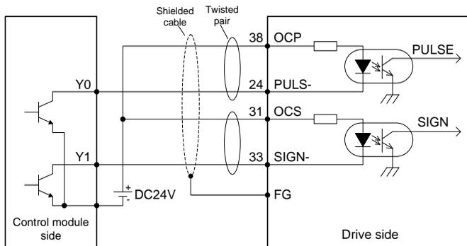
The control module is PNP type (common anode):
