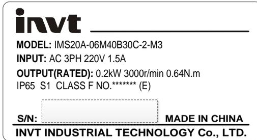
**Note:** "No.\*\*\*\*\*" in the nameplate is the motor model code (motor code for short). Please input this code into servo parameter P0.00 correctly (P0.00 is long parameter which can be set via keypad. See details at chapter 5.2.1 (8), otherwise, the servo system may not operate normally and major fault may occur to the drive and motor.
