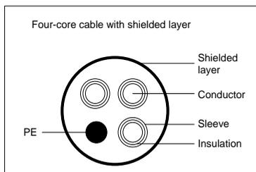
To protect the conductors, the cross-sectional area of the shielded cables must be the same as that of the phase conductors if the cable and conductor are made of materials of the same type. This reduces grounding resistance, and thus improves impedance continuity.
