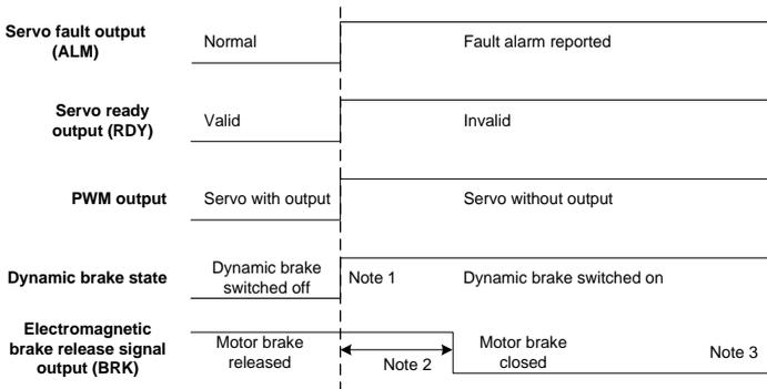
Note 1: Whether to immediately enable the dynamic brake can be set through P4.30.
