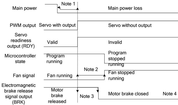
Note 1: If the voltage of the control power supply is less than 170V/330V(for 220V/400V series), the undervoltage fault will occur and the output level of the servo fault (ALM) will increase.
