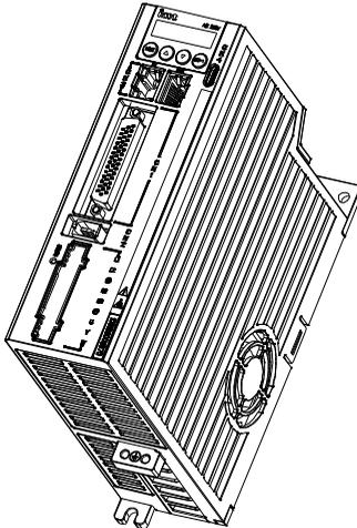
**Note:** There is a  $\varnothing 5$  installation hole at the lower left corner and upper right corner of the rear board respectively.
