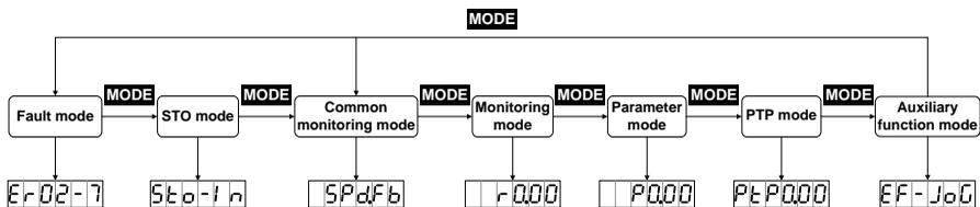
If the drive is power on, the screen will display 000000 for about 1 second, and then display 888888 for about 1 second, after that, enter into the “General monitoring mode”.
