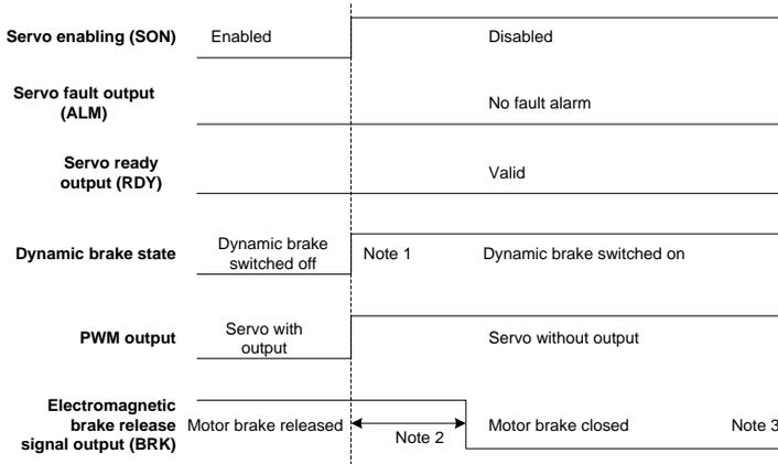
Note 1: Whether to immediately enable the dynamic brake can be set through P4.30.
