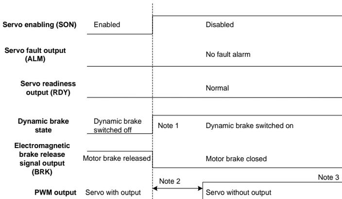
Note 1: Whether to immediately start the dynamic brake can be set through P4.30.
