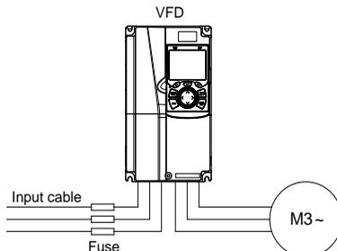
Figure 4-22 Fuse configuration
