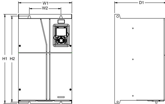
Figure C-14 Wall mounting diagram for 660V 22–132kW models
