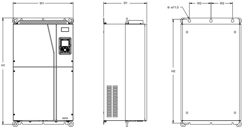
Figure C-15 Wall mounting diagram for 660V 160–220kW models
