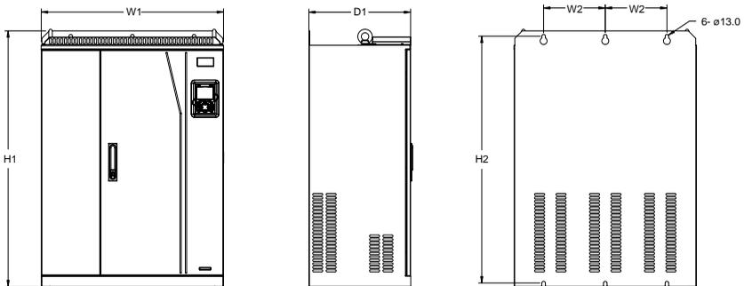
Figure C-16 Wall mounting diagram for 660V 250–355kW models
