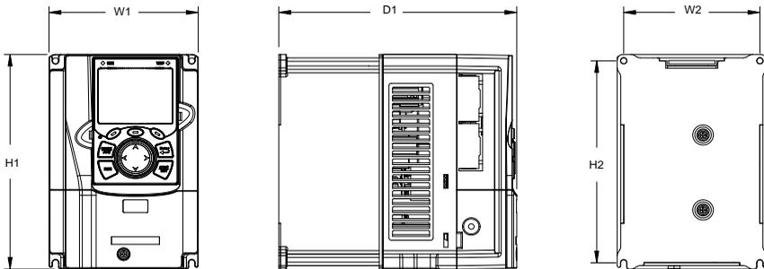
Figure C-4 Wall mounting diagram for 380V 1.5–37kW models
