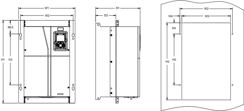
Figure C-17 Flange mounting diagram for 660V 22-132kW models
