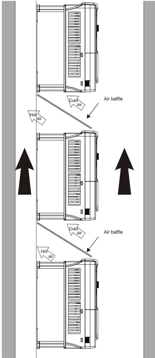
Figure 4-5 Vertical installation
