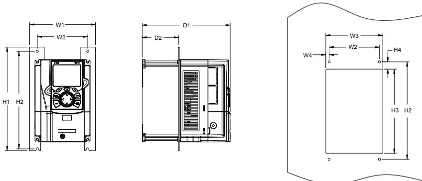
Figure C-9 Flange mounting diagram for 380V 1.5-75kW models
