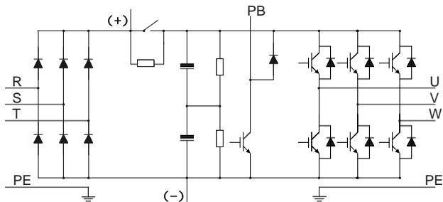
Figure 3-1 380V (15kW and lower) main circuit diagram
