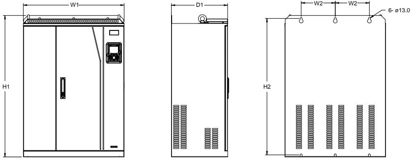
Figure C-8 Wall mounting diagram for 380V 220-315kW models
