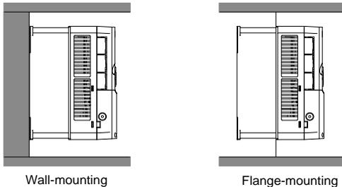
Figure 4-2 Installation mode
