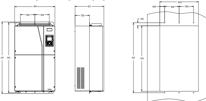
Figure C-11 Flange mounting diagram for 380V 132–200kW models
