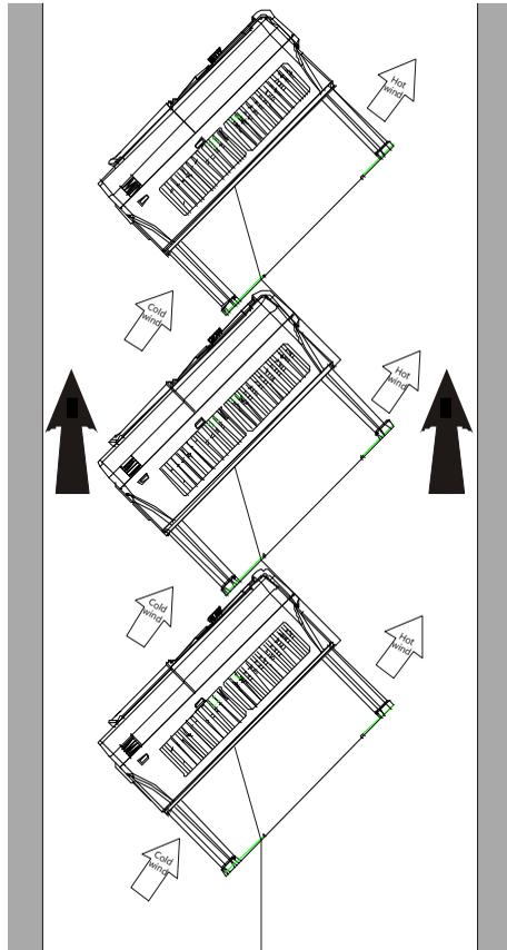
Figure 4-6 Tilted installation
