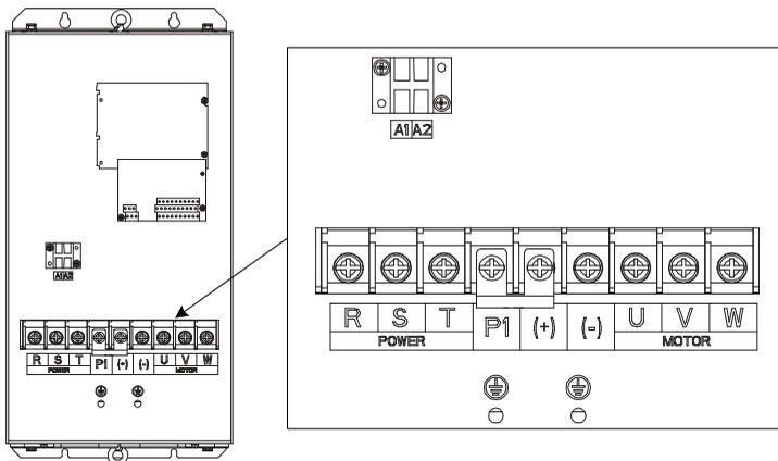
Figure 4-12 660V 22-45kW
