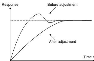
**Stabilize the feedback value as fast as possible:** when overmodulation occurred, shorten integral
