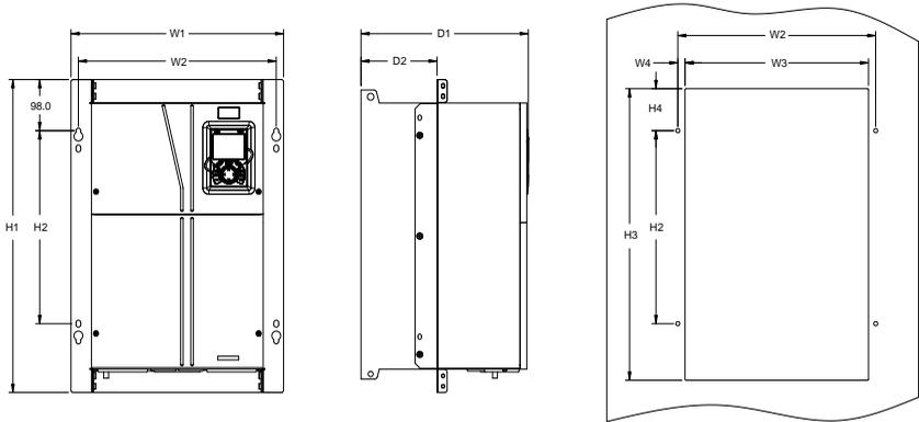
Figure C-10 Flange mounting diagram for 380V 90–110kW models
