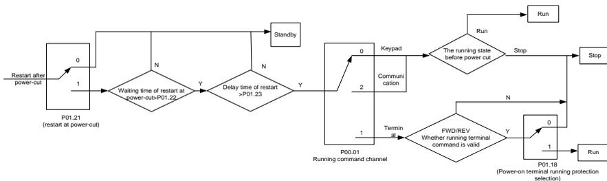
3. Logic diagram for restart after automatic fault reset
