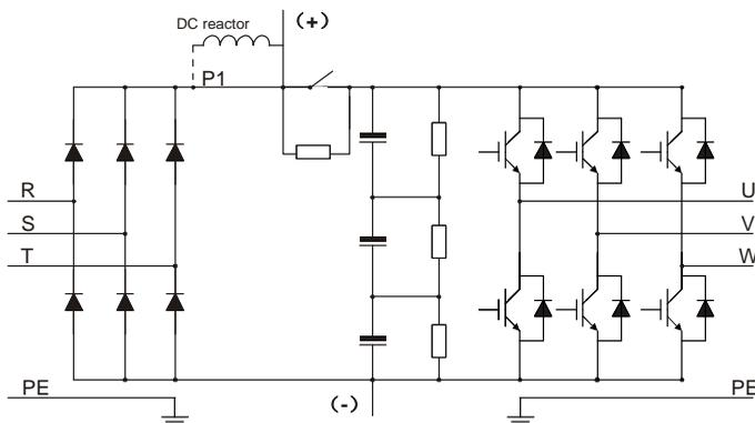
Figure 3-4 660V main circuit diagram
