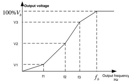
The VFD provides dedicated function codes for SVPWM control mode. You can improve the performance of SVPWM through settings.
