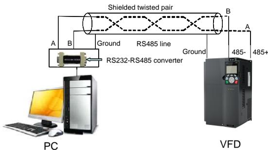
Figure 9-1 Wiring of RS485 applied to one VFD
