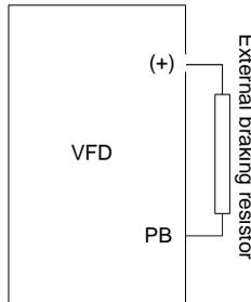
Installation of braking units
