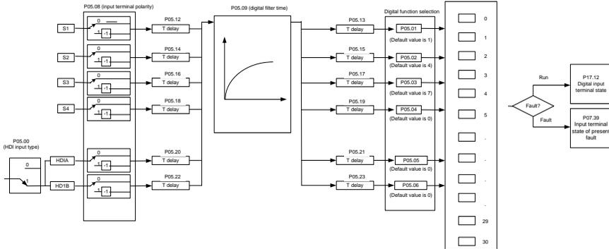
The parameters are used to set the corresponding function of digital multi-function input terminals.
