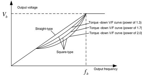
The VFD also provides multi-point V/F curve. You can alter the V/F curve outputted by VFD through setting the voltage and frequency of the three points in the middle. The whole curve consists of five points starting from (0Hz, 0V) and ending in (fundamental motor frequency, rated motor voltage). During setting, follow the rule:  $0 \leq f_1 \leq f_2 \leq f_3 \leq$  Motor fundamental frequency, and,  $0 \leq V_1 \leq V_2 \leq V_3 \leq$  Motor rated voltage
