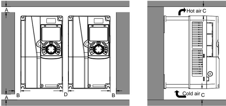
Figure 4-4 Parallel installation
