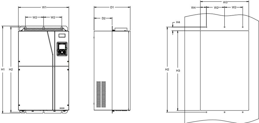
Figure C-18 Flange mounting diagram for 660V 160-220kW models
