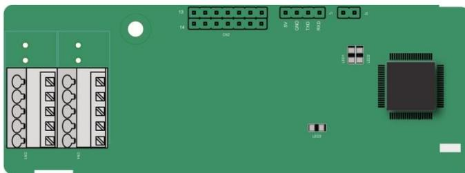
The DIP switch SW1 is used to set the voltage class (5 V or 12 V) of the power supply of the encoder. The DIP switch can be operated with an auxiliary tool.
