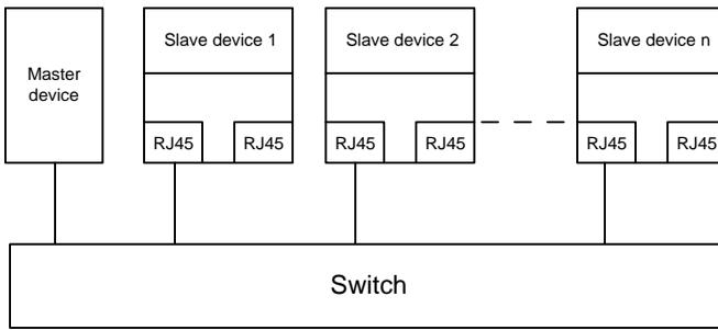
**A.6.6 EtherNet/IP communication card (EC-TX510) and Modbus TCP communication card (EC-TX515)**
