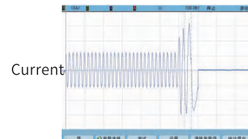
Magnetic flux braking current wave in the SVPWM mode for asynchronous motors Frequency: 50Hz Rated load: 100%
