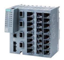
SCALANCE XC224-4C G manageable Layer 2 IE switch; IEC 62443-4-2 certified; Full gigabit; 20x 10/100/1000 Mbps RJ45 ports; 4x 1000 Mbps combo ports (either 1000 Mbps/ SFPs or 10/100/1000 Mbps RJ45 ports can be used); 1x console port; diagnostics LED; redundant power supply; temperature range -40 °C to +70 °C; assembly: DIN rail/S7 mounting rail/wall; redundancy functions; office features (RSTP, VLAN,...); PROFINET IO device; Ethernet/IP-compliant; C-PLUG slot; IEEE 1588v2 PTP
