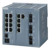
SCALANCE XB213-3LD managed layer 2 IE switch 13x 10/100 Mbit/s RJ45 ports, 3x SM FO SC-port 1x console port, diagnostics LED, redundant power supply; IEC 62443-4-2 certified; temperature range 0 °C to +60 °C; DIN-rail mounting; default PROFINET.
