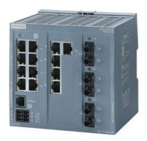
SCALANCE XB213-3 managed Layer 2 IE switch 13x 10/100 Mbit/s RJ45 ports, 3x MM FO ST port 1x console port, diagnostics LED, redundant power supply, IEC 62443-4-2 certified; temperature range 0 °C to +60 °C; DIN-rail mounting; default PROFINET.
