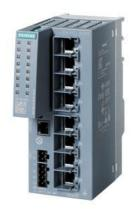
SCALANCE XC208G (E/IP) manageable Layer 2 IE switch; IEC 62443-4-2 certified; 8x 10/100/1000 Mbps RJ45 ports; 1x console port; diagnostics LED; redundant power supply; temperature range -40 °C to +70 °C; assembly: DIN rail/S7 mounting rail/wall; redundancy functions; Office features (RSTP, VLAN,...); PROFINET IO device Ethernet/IP-compliant C-plug slot; Default EtherNet/IP. IEEE 1588v2 PTP
