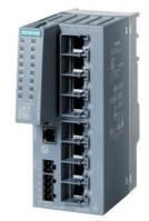
SCALANCE XC208G manageable Layer 2 IE switch; IEC 62443-4-2 certified; 8x 10/100/1000 Mbps; RJ45 ports; 1x console port; diagnostics LED; redundant power supply; temperature range -40 °C to +70 °C; assembly: DIN rail/S7 mounting rail/wall redundancy functions; office features (RSTP, VLAN,...); PROFINET IO device; Ethernet/IP-compliant; C-PLUG slot; IEEE 1588v2 PTP
