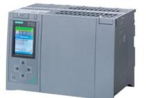
SIMATIC S7-1500H, CPU 1518HF-4 PN, central processing unit with 9 MB work memory for program and 60 MB for data, 1st interface: PROFINET RT with 2-port switch, 2nd interface: PROFINET, 3rd interface: PROFINET, 4th/5th interface: H-SYNC, SIMATIC Memory Card required
