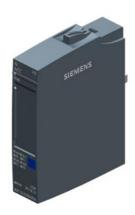
SIMATIC ET 200SP, Analog input module, AI 4xTC High Speed, suitable for BU type A0, A1, Color code CC00, channel diagnostics, 16 bit,  $\pm$ 0.1%
