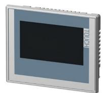
SIMATIC HMI, TP400 Basic Keyless; Basic Panel, neutral design, touch operation, 4" TFT display, 65536 colors, PROFINET interface, configurable from WinCC Basic V13/ STEP 7 Basic V13, contains open-source software, which is provided free of charge see enclosed CD
