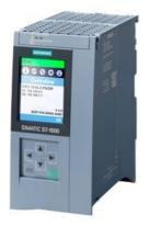
SIPLUS S7-1500 CPU 1516-3 PN/DP based on 6ES7516-3AN02-0AB0 with conformal coating, -40...+70 °C, heat sink, no PS usable, central processing unit with work memory 1 MB for program and 5 MB for data, 1st interface: PROFINET IRT with 2-port switch, 2nd interface: PROFINET RT, 3rd interface: PROFIBUS, 10 ns bit performance, SIMATIC Memory Card required
