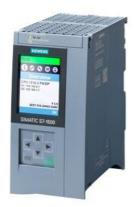
SIPLUS S7-1500 CPU 1516-3 PN/DP based on 6ES7516-3AN02-0AB0 with conformal coating, -40...+60 °C, central processing unit with work memory 1 MB for program and 5 MB for data, 1st interface: PROFINET IRT with 2-port switch, 2nd interface: PROFINET RT, 3rd interface: PROFIBUS, 10 ns bit performance, SIMATIC Memory Card required
