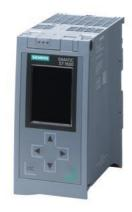
SIPLUS S7-1500 CPU 1515R-2 PN based on 6ES7515-2RM00-0AB0 with conformal coating, -40...+70 °C, start up -20 °C, heat sink, no PS usable, central processing unit with work memory 500 KB for program and 3 MB for data, 1st interface: PROFINET with 2-port switch, 2nd interface: PROFINET RT, SIMATIC Memory Card required
