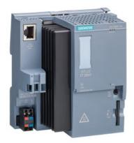
SIPLUS ET 200SP CPU 1510SP-1 PN based on 6ES7510-1DJ01-0AB0 with conformal coating, -40...+70 °C, no pluggable BusAdapter, central processing unit with work memory 100 KB for program and 750 KB for data, 1st interface, PROFINET IRT with 3-port switch, 72 ns bit performance, SIMATIC Memory Card required,
