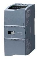
SIPLUS S7-1200 SM 1232 4AQ based on 6ES7232-4HD32-0XB0 with conformal coating, -20...+60  $^{\circ}$ C, SIMATIC S7-1200, analog output, SM 1232, 4 AQ, +/-10 V, 14-bit resolution, or 0-20 mA, 13-bit resolution
