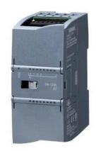
SIPLUS S7-1200 SM 1231 8AI based on 6ES7231-4HF32-0XB0 with conformal coating, -20...+60 °C, analog input SM 1231, 8 AI, +/-10 V, +/-5 V, +/-2.5 V, or 0-20 mA/4-20 mA, 12 bit+sign or (13 bit ADC)
