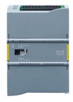
SIPLUS S7-1200 SM 1226 F-DQ 4x24VDC based on 6ES7226-6DA32-0XB0 with conformal coating, -25...+55 °C, F-DQ 4x DC 24V 2A, PROFIsafe, 70 mm width, up to PL e (ISO 13849-1)/ SIL3 (IEC 61508)
