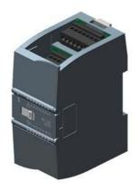
SIPLUS S7-1200 SM 1223 8DI/8DQ based on 6ES7223-1BH32-0XB0 with conformal coating, -20...+60 °C, digital input/output 8 DI/8 DQ, 8 DI 24 V DC, sink/source, 8 DQ, transistor 0.5 A
