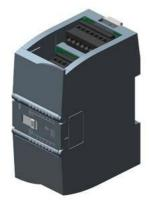
SIPLUS S7-1200 SM 1222 16DQ RLY based on 6ES7222-1HH32-0XB0 with conformal coating, -20...+60  $^\circ\text{C},$  digital output 16 DQ, relay 2 A
