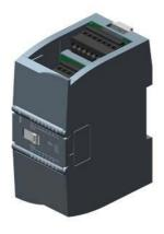
SIPLUS S7-1200 SM 1222 16DQ RLY based on 6ES7222-1HH32-0XB0 with conformal coating, -40...+70  $^{\circ}$ C, start up -25  $^{\circ}$ C, digital output 16 DQ, relay 2 A
