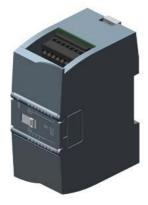
SIPLUS S7-1200 SM 1222 8DQ RLY based on 6ES7222-1HF32-0XB0 with conformal coating, -20...+60  $^\circ\text{C},$  digital output 8 DQ, relay 2 A
