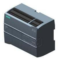
SIPLUS S7-1200 CPU 1215C DC/DC/DC based on 6ES7215-1AG40-0XB0 with conformal coating, -40...+70 °C, start up -25 °C, signal board: 0, compact CPU, DC/DC/DC, 2 PROFINET ports, onboard I/O: 14 DI 24 V DC; 10 DQ 24 V DC 0.5 A 2 AI 0-10 V DC, 2 AQ 0-20 mA DC, power supply: DC 20.4-28.8 V DC, program/data memory 125 KB
