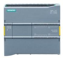
SIPLUS S7-1200 CPU 1214FC DC/DC/DC based on 6ES7214-1AF40-0XB0 with conformal coating, -25...+55 °C, compact CPU, DC/DC/DC, onboard I/O: 14 DI 24 V DC; 10 DQ 24 V DC; 2 AI 0-10 V DC, power supply: DC 20.4-28.8 V DC, program/data memory 125 KB
