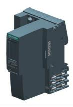
SIPLUS ET 200SP IM155-6PN ST based on 6ES7155-6AU01-0BN0 with conformal coating, -40...+70 °C, PROFINET interface module, 1 slot for BusAdapter, max. 32 I/O modules, and 16 ET 200AL modules, single hot swap, including server module (6AG1193-6PA00-7AA0)
