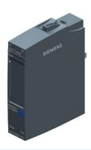
SIPLUS ET 200SP AI 4xU/I 2-w ST based on 6ES7134-6HD01-0BA1 with conformal coating, -40...+70  $^{\circ}\text{C}$ , analog input module, suitable for BU type A0, A1, color code CC03, module diagnostics, 16 bit, +/-0.3%
