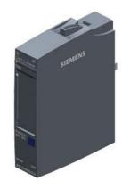
SIPLUS ET 200SP AI 2xU/I 2/4-W HF based on 6ES7134-6HB00-0CA1 with conformal coating, -40...+60 °C, analog input module, suitable for BU type A0, A1, color code CC05, channel diagnostics, 16-bit, +/-0.1%
