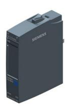
SIPLUS ET 200SP AI 4xI 2-/4-wire standard based on 6ES7134-6GD01-0BA1 with conformal coating, -40...+70  $^{\circ}$ C, analog input module, suitable for BU type A0, A1, color code CC03, module diagnostics, 16-bit, +/-0.3%
