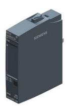
SIPLUS ET 200SP RQ 4x24VDC/2A CO ST based on 6ES7132-6GD51-0BA0 with conformal coating, -40...+70  $^{\circ}$ C, signal relay module, suitable for BU type A0, color code CC00, substitute value output, module diagnostics for: supply voltage
