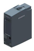
SIPLUS ET 200SP DQ 4x24..230VAC/2A HF based on 6ES7132-6FD00-0CU0 with conformal coating, -40...+70 °C, digital output module, suitable for BU type U0, color code CC20, channel diagnostics two alternative operating modes: DQ and power control,
