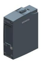
SIPLUS ET 200SP DI 4x120..230 V AC ST based on 6ES7131-6FD01-0BB1 with conformal coating, -40...+70 °C, digital input module, suitable for BU type B1, color code CC41, module diagnostics
