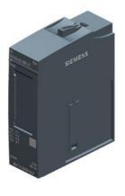
SIPLUS ET 200SP DI 8x48 V UC BA based on 6ES7131-6CF00-0AU0 with conformal coating, -40...+70  $^{\circ}$ C, digital input module, suitable for BU type U0, color code CC20, module diagnostics
