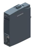
SIPLUS ET 200SP DI 16x24 V DC standard based on 6ES7131-6BH01-0BA0 with conformal coating, -40...+70 °C, digital input module, suitable for BU type A0, color code CC00, type 3 (IEC 61131) sink input, (PNP, sinking input), input delay 0.05..20 ms module diagnostics for: wire break, supply voltage
