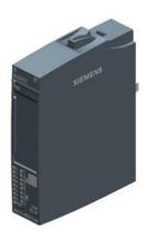
SIPLUS ET 200SP DI 8x24 V DC SRC BA based on 6ES7131-6BF61-0AA0 with conformal coating, -40...+70 °C, digital input module, suitable for BU type A0, color code CC02, source input, (NPN, sourcing input) input type 1 (IEC 61131), input delay 0.05..20 ms module diagnostics for: supply voltage
