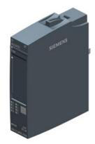
SIPLUS ET 200SP DI 8x24 V DC standard based on 6ES7131-6BF01-0BA0 with conformal coating, -40...+70 °C, digital input module, suitable for BU type A0, color code CC01, sink input, (PNP, sinking input), input type 3 (IEC 61131), input delay 0.05..20 ms module diagnostics for: short-circuit encoder supply, wire break, supply voltage
