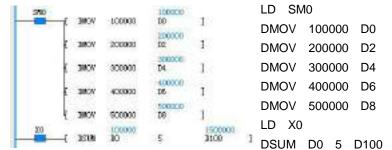
Accumulating the data of  $5\mathscr{A}$  units starting from D0, and assigning the obtained result to (D100,D101) when X0=ON.
