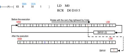
Cyclically shifting D0=2#1100110110010101 (52629) with the carry flag bit (SM181=OFF) rightward by 5 bits, and assigning the obtained result to D10 when M0=ON.In this case, D10=2#0101011001101100 (22124) and SM181=ON.
