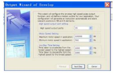
During acceleration/deceleration time, the acceleration speed of all the segments of the envelope curve is constant. For example, if the settings are as shown above, then the acceleration time taken to accelerate from 20000 Hz to 50000 Hz for the motor is:
