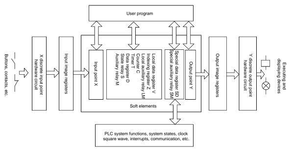
Figure 3-1 Types and functions of soft elements
