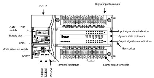
Figure 1-3 Appearance and structure of IVC3 series main modules
