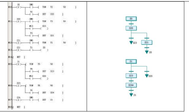
In the SFC, when the step state S0 in the first process is valid, the program can jump to the step state S23 in the second process
