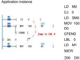
1. When the initial condition is M0=OFF and M1=ON, the CJ 0 instruction is not jumped, and D0=100. After executing the CFEND instruction, the program exits the main program in advance, instructions of LD M1 and MOV 200 D0 are not executed.
