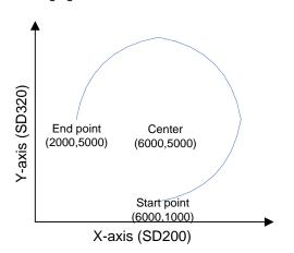
You can adopt the incremental type, the displacement of the end point to the start point is (4000, -4000), and the
