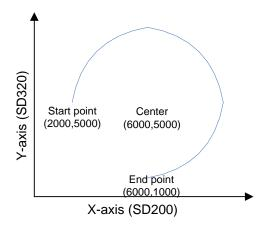
You can adopt the incremental type, the displacement of the end point to the start point is (4000, -4000), and the displacement of the center to the start point is (4000, 0). You can program like this:
