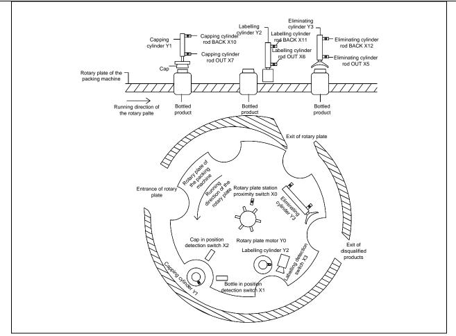
During the operation, the rotary plate rotates one step each time, which is detected by the X0 limit switch. The rotary plate stays at each step long enough for all the three procedures, driven by cylinders, finished. The cylinder rod OUT signal and cylinder rod BACK signal are monitored respectively.
