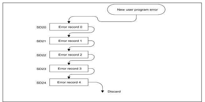
Figure 2-19 Push stack process of error codes
