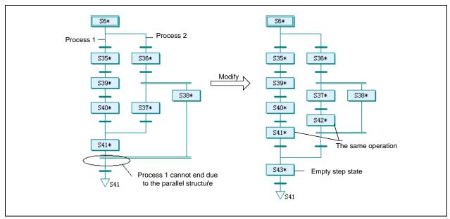
The modification method is shown in the program on the right, you need to add a step state S42 whose function is the same as S41. Then you need to add an empty step state S43 that serves as a programming structural element without actual function. The transfer conditions of S38, S41, and S43 need to be designed by the programmers, for example, all of them can adopt the transfer conditions of the original S41.
