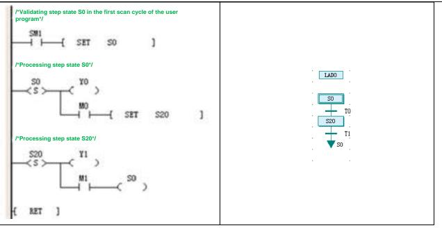
In a simple structured SFC program, when the step transfer conditions are met, the program is sequentially transferred from the current step state to the next step state without any branch structure. At the last step, when the transfer conditions are met, the SFC program section either ends or transfers to the initial step state.
