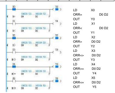
Conducting the comparison on (D0,D1) and (D2,D3), and using the comparison result in parallel connection with other nodes to determine the output state of the subsequent elements.
