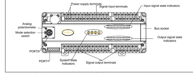
Figure 1-2 Appearance and structure of IVC2L series main modules
