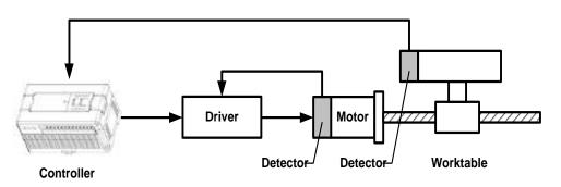
Figure 11-4 Closed-loop control systemdiagram
