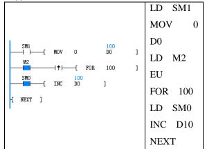
The initial conditions of the operation are: D0=0, and M2=OFF. When M2 changes from OFF to ON, the instructions within the FOR-NEXT structure are consecutively executed for 100 times. D0 is increased by one for 100 times. When the cycle is over, D0=100.
