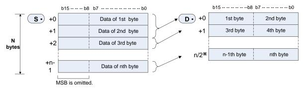
2. When S2 is odd, the least significant byte that is combined finally is cleared.
