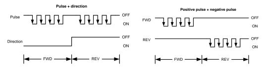
Figure 11-7 Definition of pulse output form
