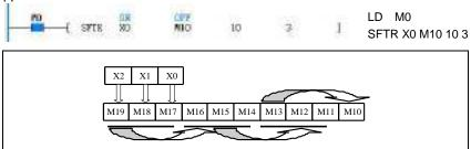
1. Shifting the content of 10 units starting from M10 rightward by 3 units, discarding M10 to M12 on the rightmost end, and shifting the content of 3 units starting from X0 to the left end of the bit string when M0=ON.
