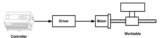
Figure 11-3 Open-loop control system diagram
