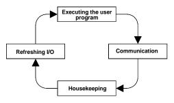
Figure 2-1PLC operating mechanism
