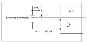
4. With the large load current, the OFF time of the transistoris relatively long. When executing the PWM, PLSY and PLSR instructions, it is required the output port of the transist or be connected to the corresponding load. When the output waveform does not conform to the instruction operand, it is viable to increase the load current of the transistor (the transistor load≤100mA).
