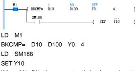
When M1=ON, the contents of the four units starting from D10 are compared with the contents of the four units starting from D100, and the result is stored in the four units starting from Y0. In addition, when the comparison result is all ON, Y10 turns ON.
