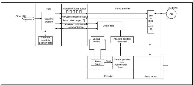
Figure 11-1 Absolute position system function diagram
