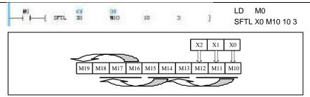
1. Shifting the content of 10 units starting from M10 leftward by 3 units, discarding M17 to M19 on the leftmost end, and shifting the content of 3 units starting from X0 to the right end of the bit string when M0=ON.
