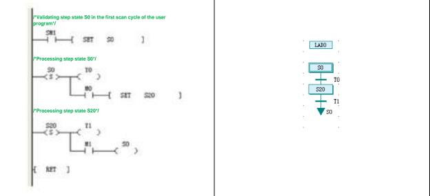
Figure 4-3 Application instance of SFC
