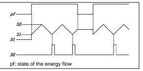
The execution process of a triangle wave instruction is shown as follows (**S3**=5).
