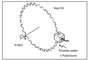
1. Counting the input pulse designated by X0 within 1000ms, and storing the count result to the storage unit of D10 when M0 is ON, in which D11 is the current count value within 1000ms, and D12 is the elapsed time within 1000ms.
