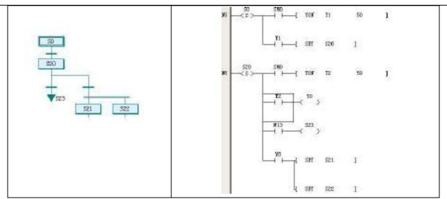
The state of S elements is switch between ON and OFF according to the transfer conditions, thus making the program transfer from one step state to another. When a S element changes from ON to OFF, the output elements of the corresponding step state are reset or cleared. For details, refer to section 5.3.1 "STL: SFC state loading instruction".
