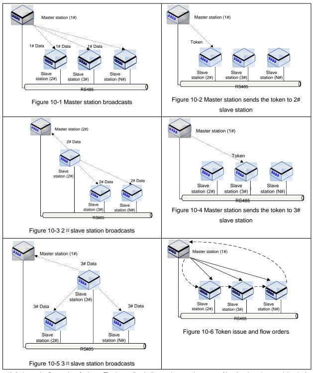
Figure 10-6 shows the flow order of tokens. The heavy line indicates the actual process of issuing the token, and the dashed line indicates the order of the station in which the token is held and broadcasted. You need to note that the token is not passed by one slave station(such as 2#PLC) to another slave station (such as 3#PLC), but the token is first issued by the master station to 2#PLC, and then issued by the master station to 3# PLC.
