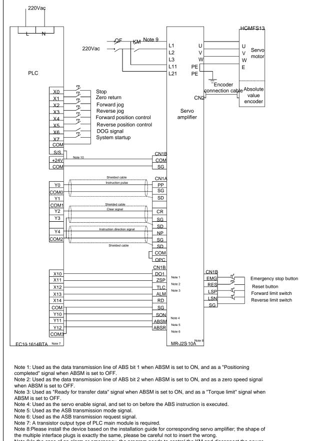
Note 9:In the case of an alarm or emergency, the program needs to control the KM and disconnect the power supply.
