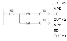
1. In two consecutive scan cycles, the states of M2 contact are OFF and ON respectively, and the EU instruction detects a rising edge change, so that Y2 outputs an ON state with a scancycle width.
