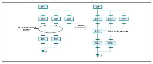
In the left diagram below, the selection merge is connected immediately with a parallel branch structure, which is prohibited too. You can also modify it by adding an empty step state as shown in the right diagram.
