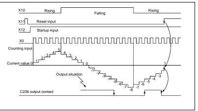
1. Initializing the hardware counter corresponding to C236 when X12 changes from OFF to ON. X0 is the pulse input end of C236 while C236 counts the external pulse of X0. X0 is a general input point when X12 is OFF, and C236 cannot count the external pulse of X0.
