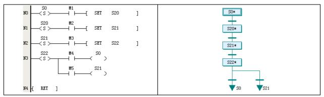
In the SFC, when the step state S22 is valid and one of the transfer conditions is met, the program jumps to S21 and re-run the step state S21. Under another transfer condition, the program jumps to the initial step state S0 and re-run allstep states.
