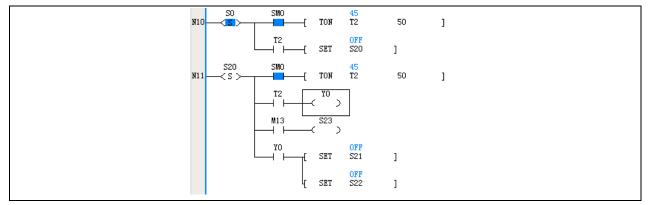
5. Failing to interlock the soft elements
