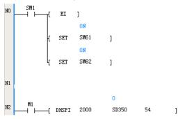
The interrupt number of the interrupt subprogram can be set to 54 or other position-based interrupt source of high-speed output, and then the program to be executed when passing the position can be written in the interrupt subprogram.
