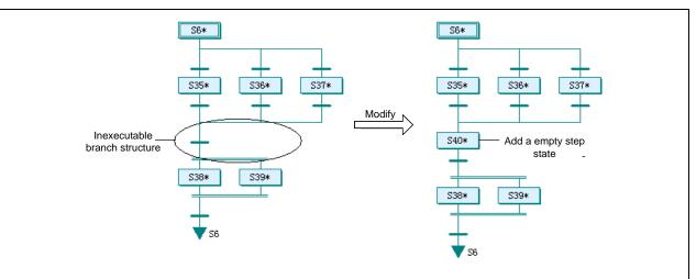
You can address other tricky structures, such as parallel merge connected with parallel branches, or parallel branches connected with selection branches, by adding an empty step state.
