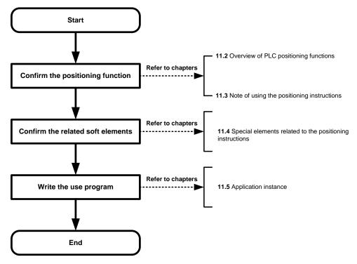
Figure 11-6 Process of positioning control
