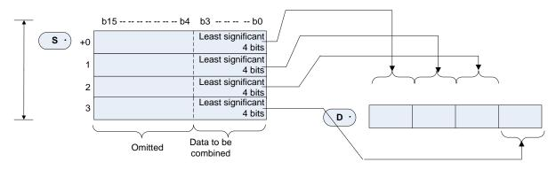
2. When S2 is ranging from 1 to 3, the ones of the LSB {4 × (4 - S2)} of D are zero.
