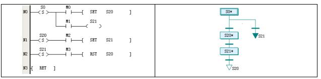
In the SFC program shown in the preceding figure, the jump symbol S21 is used as the jump, while the step state S20 is skipped. In fact, a branch structure is selected before the jump is performed.
