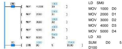
Accumulating the data of 5 units starting from D0, and assigning the obtained result to (D100,D101) when X0=ON.In this case, (D100,D101)=D0  $+\ldots$ +D4=15000.
