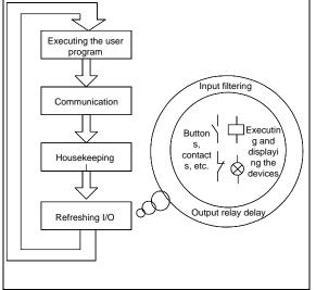
Figure 3-2 Schematic diagram of I/O refresh
