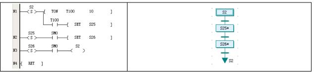
As shown in the LAD program, the step state S2 starts with a STL instruction, and the following TON instruction is the internal instruction sequence of S2. An internal instruction of the step state can be made up of multiple statements, which is actually a relatively complete program section, and almost consistent with the normal LAD counterpart.
