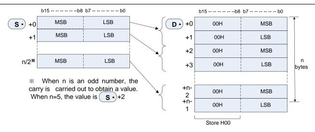
2. When S2 is odd, only the high byte (8 bits) is the object data in the last data of the separated source. For example, when n=5, the data of the low bytes of S - S+2 are stored in D - D+4.
