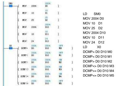
Conducting the BIN comparison on the date data starting from D0 and D10 respectively, and assigning the comparison result to the destination data (M0, etc.).
