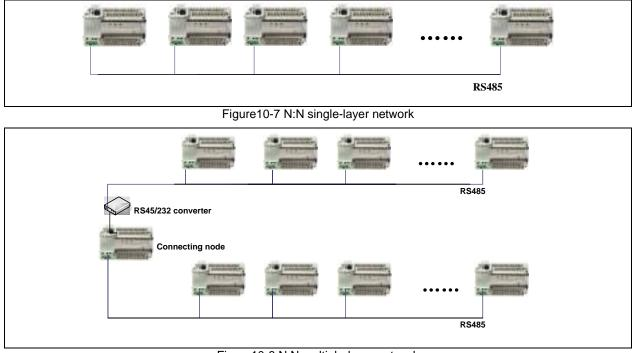
Figure10-8 N:N multiple-layer network
