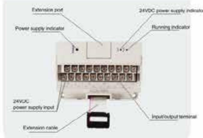
**Communication extension module****CANopen master module: IVC2L-COPM**
