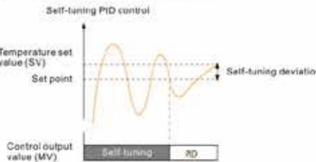
Autotuning, adaptation, automatic generation of PID parameters;
