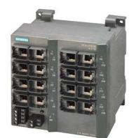
SCALANCE X216, managed IE switch, 16x 10/100 Mbit/s RJ45 ports, LED diagnostics, error-signaling contact with set pushbutton, redundant power supply, PROFINET IO device, network management, redundancy manager integrated, incl. electron. manual on CD-ROM, C-PLUG optional.
