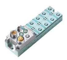
SIMATIC DP, Basic module BM 141 ET 200ECO: 8 DI 24 V DC; 8xM12, single assignment, Degree of protection IP65/67; Connection block 6ES7194-3AA00-0.A0 separately order
