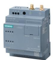
LOGO! CMR2020 communication module for connection LOGO! 8 to GSM/GPRS network; 1 RJ45 port for Ind. Ethernet connection to LOGO! 8; 2xDI; 2xDO; write/read access to LOGO! variables; SMS dispatch/ receiving of text messages; email dispatch; position detection GPS; time synchronization/ forwarding with real time clock; Configuration/diagnostics via web interface; Remote access via OpenVPN/HTTPs, DynDNS; Observe national approval! Manual available as a download .
