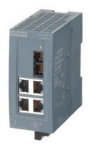
SCALANCE XB004-1 unmanaged Industrial Ethernet Switch for 10/100 Mbit/s; for setting up small star and line topologies; LED diagnostics, IP20, 24 V AC/DC power supply, with 4x 10/100 Mbit/s twisted pair ports with RJ45 sockets; 1 x 100 Mbit/s multimode glass fiber-optic cable port with SC socket; manual available as a download .
