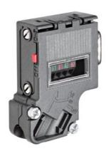
PROFIBUS bus connector, RS 485, screw, without programming port, 35° SIMATIC DP, Connection plug for PROFIBUS up to 12 Mbit/s with inclined cable outlet, 15.8x 54x 39.5 mm (WxHxD), terminating resistor with isolating function, without PG socket
