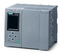
SIMATIC S7-1500F, CPU 1517F-3 PN/DP, Central processing unit with Work memory 3 MB for Program and 8 MB for data, 1st interface: PROFINET IRT with 2-port switch, 2nd interface: PROFINET RT, 3rd interface: PROFIBUS, 2 ns bit performance, SIMATIC Memory Card required
