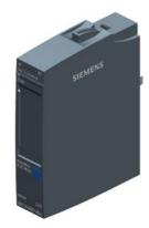
SIMATIC ET 200SP, ANALOG INPUT MODULE, AI 4XI 2-/4-WIRE STANDARD, PACKING UNIT: 1 PIECE, FITS TO BU-TYPE A0, A1, COLOR CODE CC03, MODULE DIAGNOSIS, 16BIT, +/-0,3%
