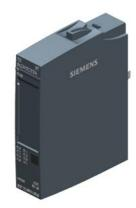
SIMATIC ET 200SP, Digital output module, DQ 8x 24V DC/0,5A Standard, Source output (PNP,P-switching) Packing unit: 1 piece, fits to BU-type A0, Colour Code CC02, substitute value output, module diagnostics for: shortcircuit to L+ and ground, wire break, supply voltage
