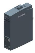
SIMATIC ET 200SP, Digital input module, DI 8x 24V DC Basic, type 2 (IEC 61131), sink input, (PNP, P-reading), Packing unit: 1 piece, fits to BU-type A0, Colour Code CC01, input delay time 0,05..20ms, module diagnostics for: supply voltage
