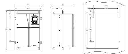
Figure C-10 090G/110P-110G/132P flange installation diagram
