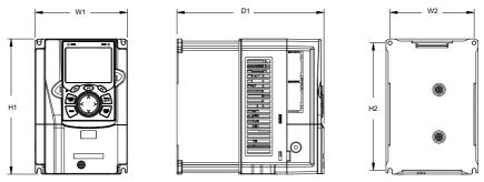
Figure C-4 1R5G/2R2P-037G/045P wall-mounting diagram
