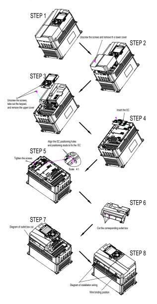
Figure A-3 Expansion card installation process diagram
