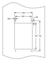
Figure C–9 1R5G/2R2P-075G/090P flange installation diagram
