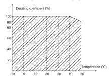
**Note:** It is not recommended to use the VFD at a temperature higher than 50°C. In case of violation, we shall bear no liability for the consequences caused.
