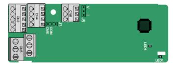
CME and COM are shorted through J3 before delivery, and J5 is the jumper for selecting the output type (voltage or current) of AO2.
