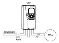
Figure 4–19 Fuse configuration
