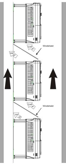
Figure 4-5 Vertical installation
