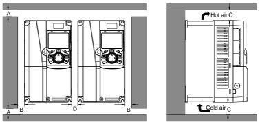
Figure 4-4 Parallel installation
