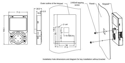
Figure C–1 Keypad structure diagram
