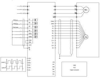
The following figure shows the external wiring of the PG card when it is used in combination with an
