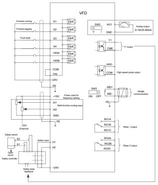
Figure 4–15 Control circuit wiring diagram
