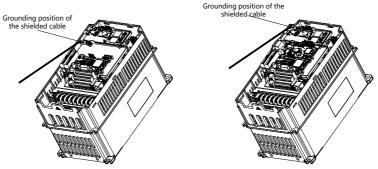
Figure A-4 Expansion card grounding diagram
