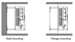
Figure 4-2 Installation mode
