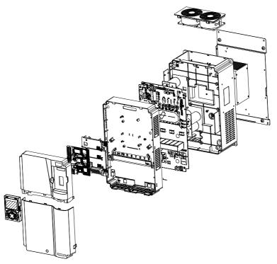
Figure C-3 VFD structure diagram
