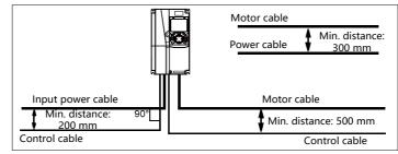
The following figure shows the cable arrangement distance requirements.
