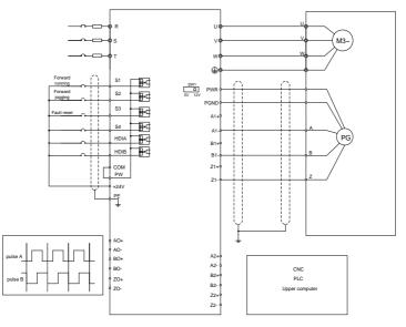
The following figure shows the external wiring of the expansion card used in combination with a differential encoder.
