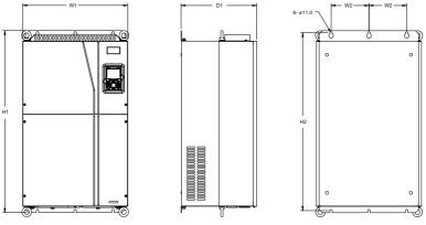
Figure C-7 132G/160P-200G/220P wall-mounting diagram
