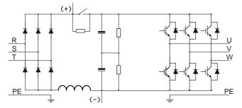
Figure 3–3 Main circuit diagram for 045G/055P–110G/132P
