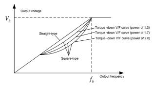
The VFD also provides multi-point V/F curves. You can change the V/F curves output by the VFD by setting the voltage and frequency of the three points in the middle. A whole curve consists of five points starting from (0Hz, 0V) and ending at (motor fundamental frequency, motor rated voltage).
