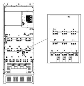
Figure 4–13 Main circuit terminal diagram for 355G/400P–500G models
