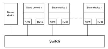
A.6.6 EtherNet/IP communication card (EC-TX510) and Modbus TCP communication card (EC-TX515)
