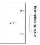
Installation of braking units:
