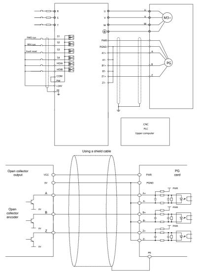
The following figure shows the external wiring of the PG card when it is used in combination with a push-pull encoder.
