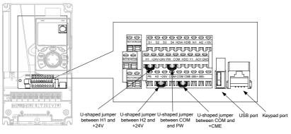
Figure 4–16 Position of U-type short connector
