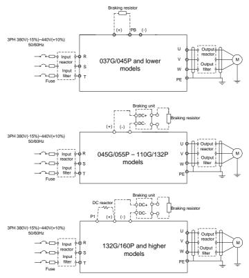
Figure 4–7 Main circuit wiring diagram
