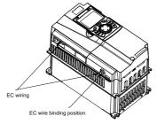
Figure A-5 Expansion card wiring
