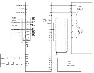
The following figure shows the external wiring of the expansion card used in combination with a push-pull encoder.
