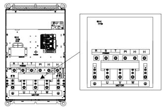
Figure 4–11 Main circuit terminal diagram for 132G/160P–200G/220P models
