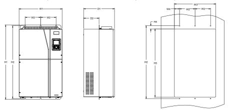
Figure C–11 132G/160P-200G/220P flange installation diagram
