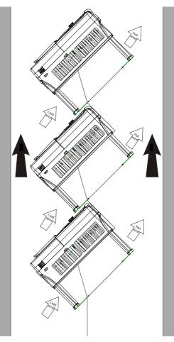
Figure 4-6 Tilted installation
