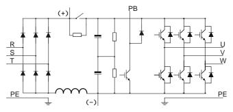
Figure 3-2 Main circuit diagram for 018G/022P-037G/045P
