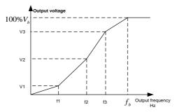
The VFD provides dedicated function codes for the space voltage control mode. You can improve the space voltage control performance by means of setting.
