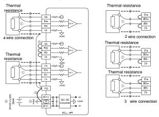
Figure 1-4 Wiring of IVC1-4PT user port
