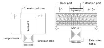
Figure 1-1 IVC1-4PT appearance Figure 1-2 IVC1-4PT ports
