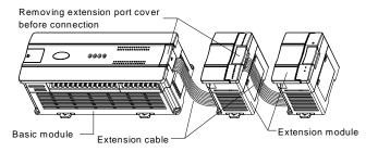
Figure 1-3 Connecting into system
